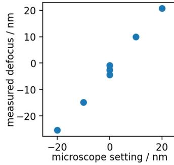
**Fig 2.** : Plot of the fitted defocus vs. the nominal one set at the microscope.
