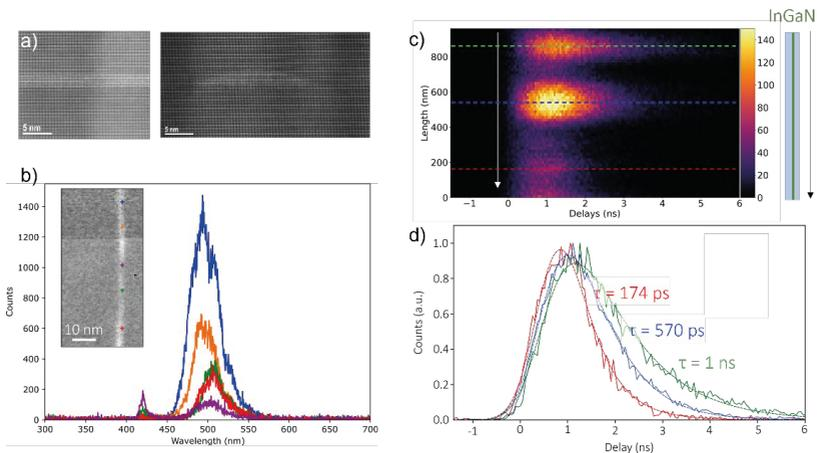
**Figure 1.** a) STEM-HADF image of an  $\text{In}_{0.3}\text{Ga}_{0.7}\text{N}/\text{GaN}$  quantum well. b) Cathodoluminescence spectra at different position of along the quantum well. EHT = 100 keV at nitrogen temperature. c) Decay map along the quantum well with different decay depending on the position of the electron beam. d) Decay trace extracted from c) with the corresponding lifetimes extracted using a mono-exponential model.
