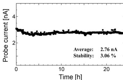
**Fig 2.** Stability of the probe current for 24 hours
