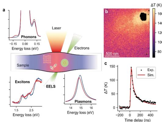
**Figure 1.** Description of the photon-electron pump-probe experiment.
