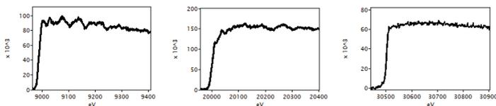
Figure 1. From left to right: Cu K-edge, Mo K-edge and Sb K-edge
