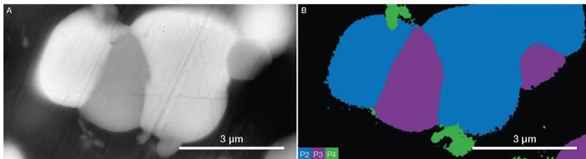
**Figure 1.** AA2024 sample subjected to the T3 aging treatment. Various intermetallic particles are differentiated through a combination of backscattered electron contrast imaging (A) and ChemiPhase analysis (B).
