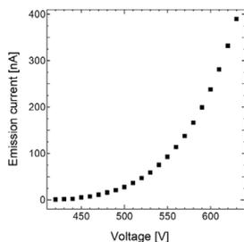
**Fig 1.** Filed emission I-V curve
