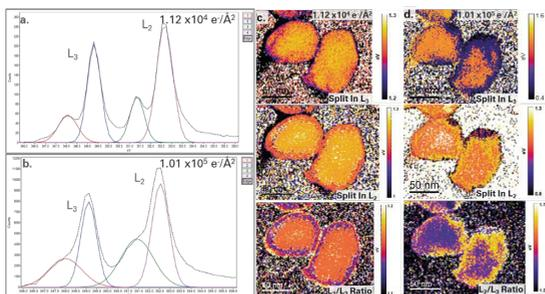
**Figure 1.** (a) Extracted Ca L<sub>2,3</sub> ELNES (Edge) from pristine CaCO<sub>3</sub> (b) and after a total dose of 1.01e5 e-/Å<sup>2</sup>. Gaussian functions were fitted to each peak (1-4) using NLLS fitting. The split in the L<sub>3</sub> and the L<sub>2</sub> edges, as well as the L<sub>2</sub>/L<sub>3</sub> edge intensity ratio, are calculated in (c,d) using the fitted parameters from Gaussians shown in (a).
