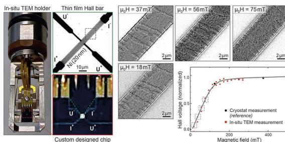
**Fig. 1.** Protochips Fusion Select holder with home-made measurement chip. LTEM images recorded simultaneously with Hall measurements reveal the domain growth upon magnetizing a 20 nm Ni film.
