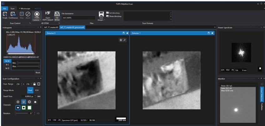
**Fig 1.** Screenshot of EMplified Scan showing virtual dark and bright field detector images of a cross section of sputtered InP. The monitor image (right lower corner) shows the live diffraction pattern on a TemCam-XF416.
