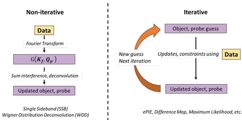
Figure 1. Simplified workflows for (a) non-iterative and (b) iterative electron ptychography.
