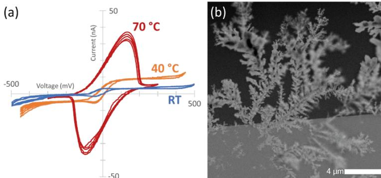
**Fig 1.** (a) Chemical redox cycling of 50 mM ferric and 50 mM ferrous chloride at room temperature (blue), 40 °C (orange) and 70 °C (red) within a closed-cell TEM system. (b) TEM micrograph of silver dendrites formed in real time on the platinum working electrode by chronoamperometry.
