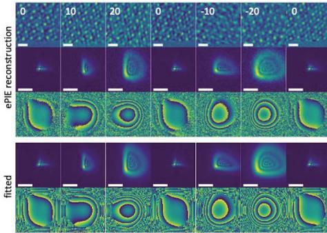
**Fig 1.** : Top: Phase grating (top) with foci (nm), probe (middle), aberration function (bottom) from ePIE. Bottom: Probe fit.
